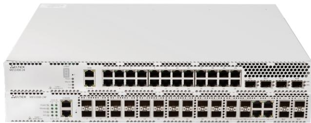
The new generation switches can be used in service provider networks as aggregation or transport switches. They ensure high performance due to the interfaces operating at speeds of 10 Gbps or 1 Gbps. MES aggregation switches feature set includes L2 functions, static routing, dynamic routing, stacking of up to 8 devices, redundant and hot-swappable power supplies.
