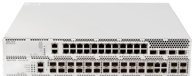
The new generation switches can be used in service provider networks as aggregation or transport switches. They ensure high performance due to the interfaces operating at speeds of 10 Gbps or 1 Gbps. MES aggregation switches feature set includes L2 functions, static routing, dynamic routing, stacking of up to 8 devices, redundant and hot-swappable power supplies.
