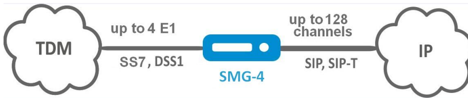
Fig. 1.1—Interfacing of TDM and VoIP Network Signalling and Media Streams Using SMG-4
