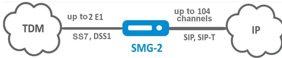
Fig. 1.2—Interfacing of TDM and VoIP Network Signalling and Media Streams Using SMG-2
