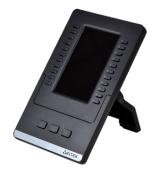
VP-EXT22 — console that extends functionality of the VP-20(P) and VP-30P(-WB) IP-phones. The device includes 22 additional keys with LED indication, color LCD, and 3 virtual pages, which increase the number of programmable keys up to 66.
