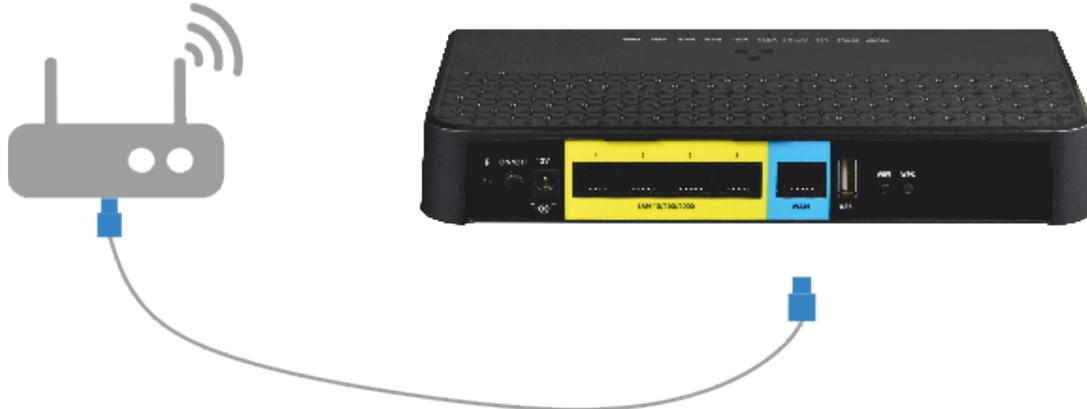
**⚠ If the third-party router uses the 192.168.1.0/24 subnet, then when connecting RG-5520G-Wax/Wax-Z its LAN address will automatically change to 192.168.2.1.**
