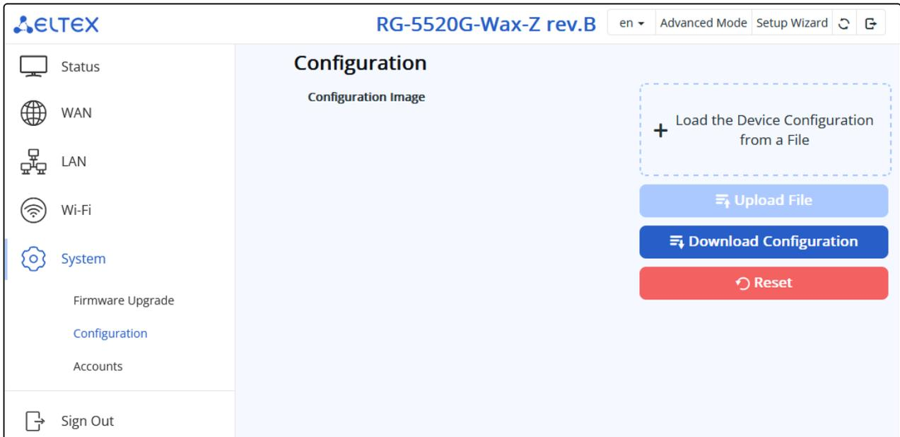
**Configuration Image** – selection of the configuration file saved on the local computer. To update the device configuration, click the "Load the Device Configuration from a File" button, select the file (in .cfg format) and click the "Upload File" button.
