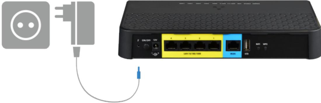
2. Connect the Ethernet cable provided by the Internet service provider to the WAN connector or the 4G modem to the USB port of the router. As soon as the **Status** indicator stops flashing and lights constantly, the connection to the provider's network is established.
