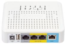
**TAU-1M.IP** is a VoIP gateway with an embedded router. The device has an FXS port and two 10/100Base-T LAN ports for PC or set-top boxes connection. The gateway is connected to service provider networks via a 10/100Base-T WAN port and has a USB port for 3G/4G modems or USB storage devices.
