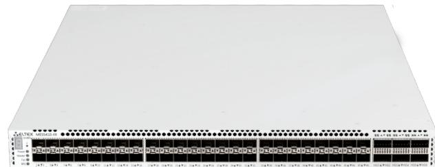
**MES5410-48** switches are high performance devices with 25GBASE-R and 100GBASE-R interfaces that can be used as aggregation switches in carrier networks and as Top-of-Rack or End-of-Row switches for data centers.
