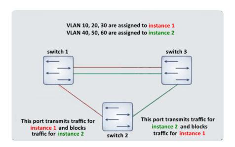
Figure A.1 — Configuring the Spanning Tree protocol
