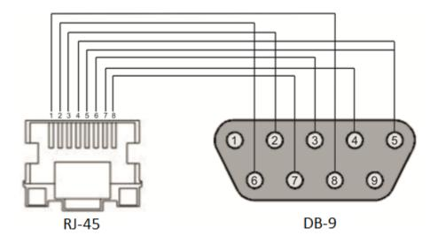
Figure B.1 — Console cable connection
