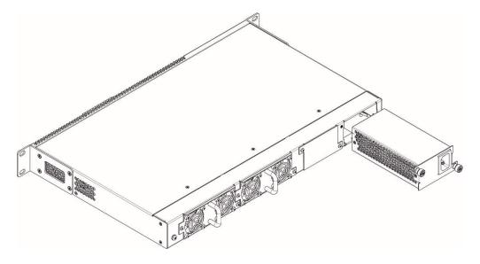
Figure 45 — Power module installation
