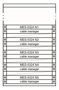
Figure 44 - MES5324 switch rack installation
