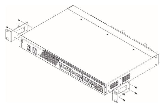
Figure 42 — Support brackets mounting
