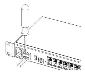
Figure 46 — Connecting the battery to the device
