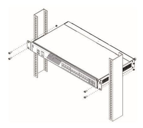
Figure 43 — Device rack installation
