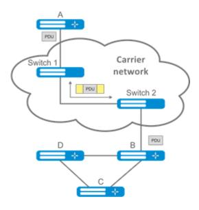
Figure 52 — L2PT function operation example
