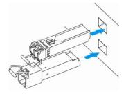
Figure 47 — SFP transceiver installation
