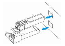
Figure 50 — SFP transceiver removal
